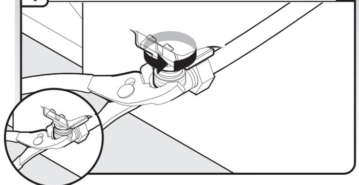
Be sure rubber washer is properly seated in fitting. Slide the  $\frac{3}{4}$ " fitting up to the valve and hand tighten to avoid unintentional cross-threading. Hand tighten until the coupling is tight. Using pliers, check the tightness of the coupling. An additional  $\frac{1}{4}$  to  $\frac{1}{2}$  turn may be required to seal the rubber gasket.
